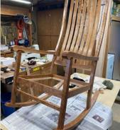
The rockers and back slats are steam-bent laminations. The back legs and arms were rough-cut on a bandsaw and cleaned up using a template on a router table. The biggest challenge was cutting the pieces for the laminations - the wood was highly figured in one orientation (you can see that in the wavy pattern along the back legs), so the pieces tended to chip out when I ran them through the planer that way. I had to cut new pieces in the other orientation to get them through the planer.
