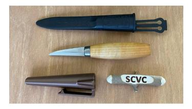
Pranay 3D printed nice sheaths for Morakniv wood carving knives. The original sheath for those knives (at the top of the picture) is too long. The 3D-printed sheath fits snugly and helps save space in a woodcarving toolbox.
